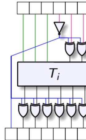
We exploit symmetry to trade one table input bit for two rows of XOR gates...
